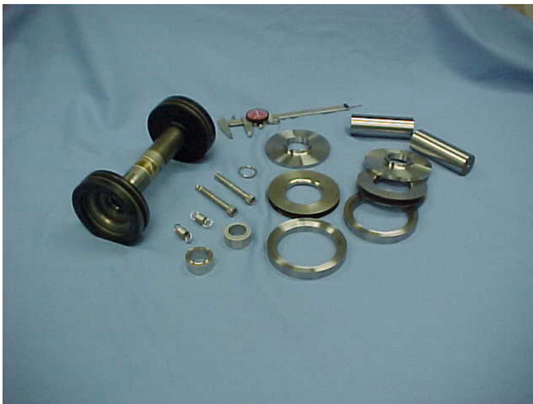
Figure 4: The details that make up a Torque Tube Assembly
